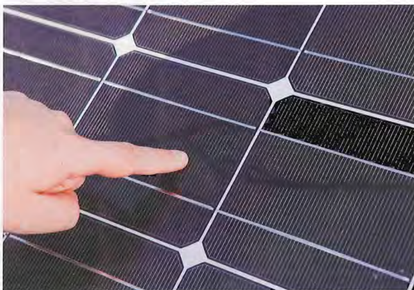
Snail tracks: These finger-thick dark lines crisscrossing solar cells result from a chemical reaction. The cause and effects of the reaction are still being researched.
