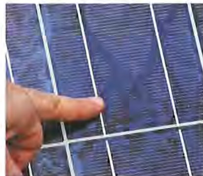
Most of the operators who reported snail tracks to PHOTON did not observe any impact on the output of their modules. But Javier Hernández from Ingeniería Medioambiental Helios in Spain says that his system's yield has fallen by around 20 percent. CSI, the manufacturer, has not taken any remedial action to date.
